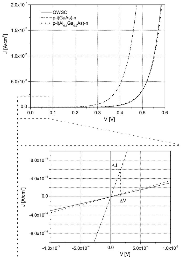
Fig. 4. Dark J-V characteristics for shunt resistance of p-i-n and QWSC calculation.
