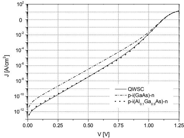
Fig. 2. Dark J-V characteristics of QWSC, p-i(GaAs)-n and p-i( $\text{Al}_{0.1}\text{Ga}_{0.9}\text{As}$ )-n structures.
