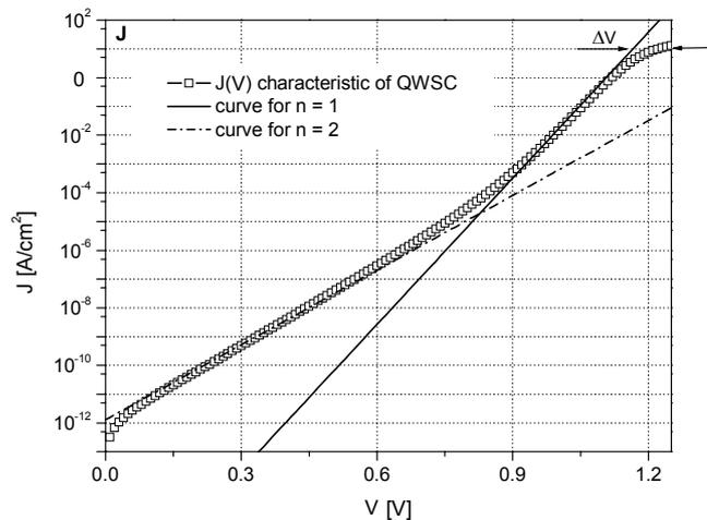
Fig. 3. Emission coefficients and series resistance evaluation of 2QWSC.
