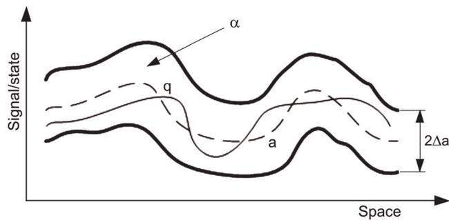
Fig. 1. The output of the SPM measurements presented by a corridor  $2\Delta a$  (doublet measurement error).
