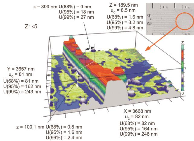
Fig. 2. The result of the C-AFM measurement of the sample topography [16].
