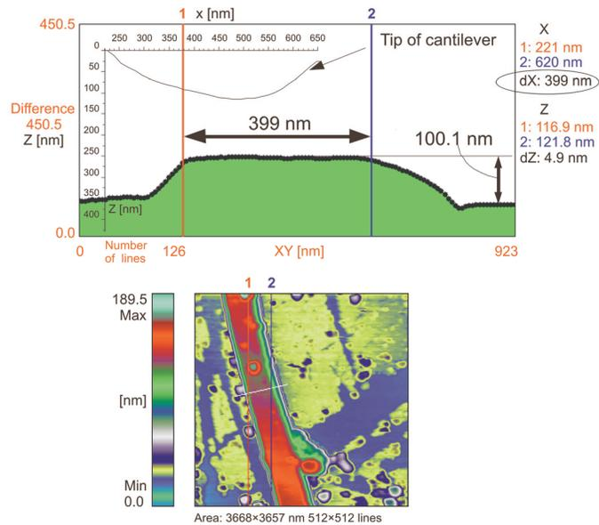
Fig. 3. Scheme of the measured profile [16].
