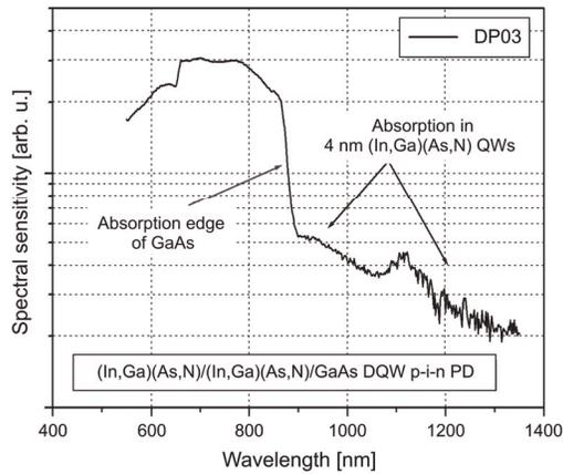
Fig. 6. Spectral characteristic of (In, Ga)(As, N)/(In, Ga)(As, N)/GaAs DQW p-i-n photodetector.
