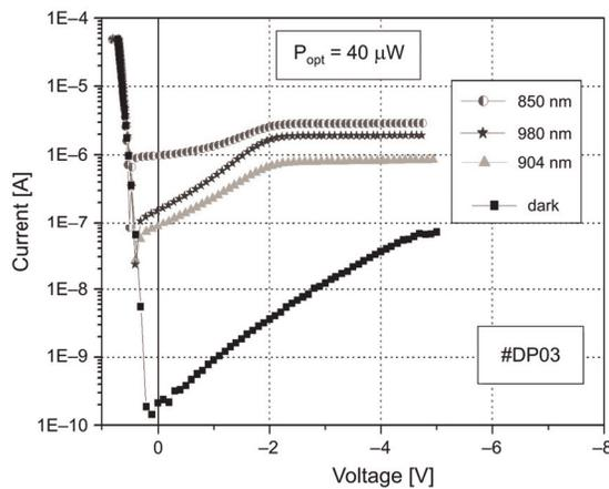
Fig. 5. Current-voltage characteristic of  $(\text{In,Ga})(\text{As,N})/(\text{In,Ga})(\text{As,N})/\text{GaAs}$  DQW p-i-n photodetectors (#DP03) for different wavelengths.
