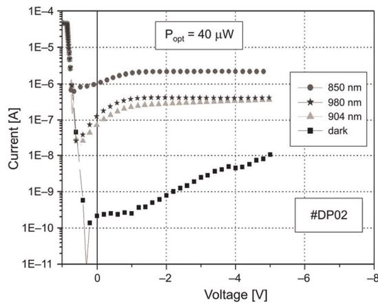
Fig. 4. Current-voltage characteristic of Ga(As,N)/GaAs DQW p-i-n photodetectors (#DP02) for different wavelengths.
