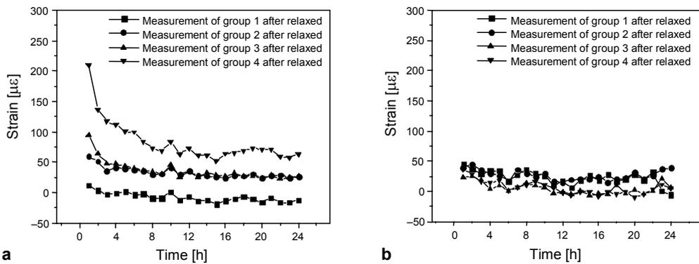
Fig. 12. Strain values of the Type-A (a) and Type-B (b) changed with time within 24 hours after being relaxed from constant length stretching.
