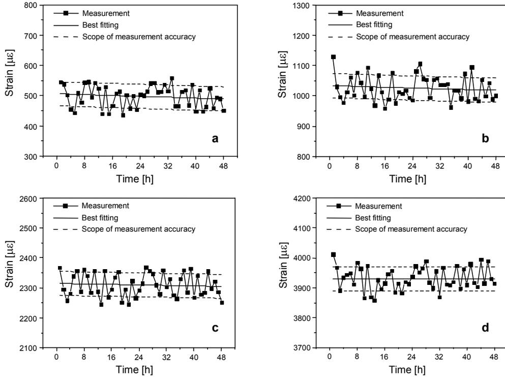
Fig. 11. Strain value of the Type-B changed with time under constant length stretching, 500 $\mu\epsilon$  (a), 1000 $\mu\epsilon$  (b), 2000 $\mu\epsilon$  (c) and 4000 $\mu\epsilon$  (d), within 48 hours.
