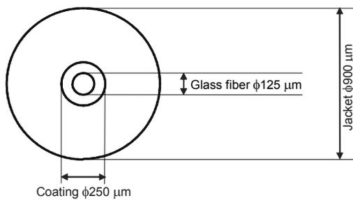
Fig. 1. Structure of optical fiber.
