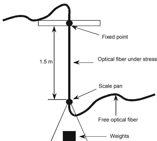
Fig. 2. Laboratory rack for constant load stretching of optical fiber.
