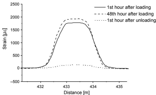
Fig. 4. Strain distribution lines of the Type-A under constant load stretching.
