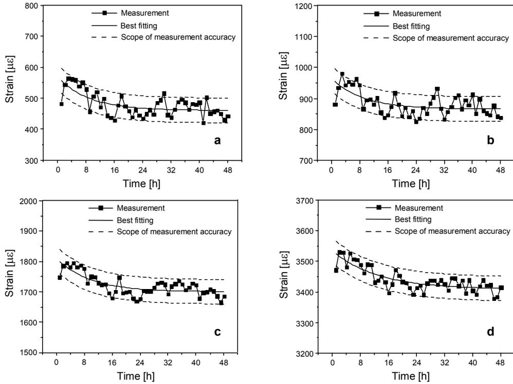
Fig. 9. Strain value of the Type-A changed with time under constant length stretching, 500 $\mu\epsilon$  (a), 1000 $\mu\epsilon$  (b), 2000 $\mu\epsilon$  (c) and 4000 $\mu\epsilon$  (d), within 48 hours
