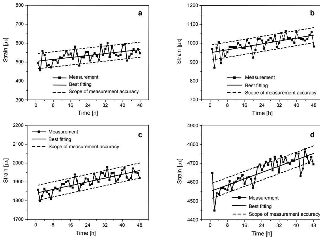
Fig. 5. Strain value of the Type-A changed with time under constant load stretching, 50 g (a), 100 g (b), 200 g (c) and 500 g (d), within 48 hours.
