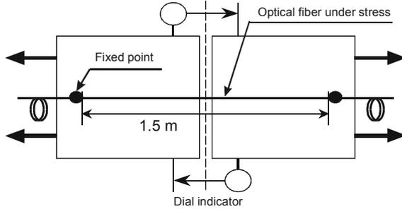
Fig. 3. Laboratory table for constant length stretching of optical fiber.
