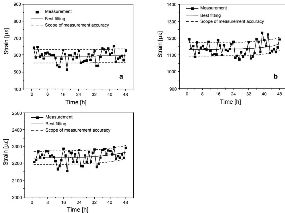
Fig. 7. Strain value of the Type-B changed with time under constant load stretching, 50 g (a), 100 g (b) and 200 g (c), within 48 hours.
