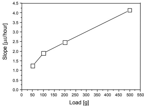
Fig. 6. Slope of the curves in the experiment for constant load stretching within 48 hours.
