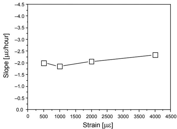
Fig. 10. Slope of the curves in the experiment for constant length stretching within 48 hours.
