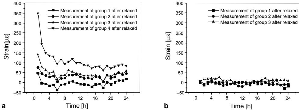
Fig. 8. Strain values of the Type-A (a) and Type-B (b) changed with time within 24 hours after being relaxed from constant load stretching.
