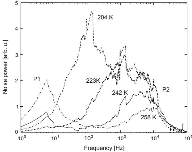
Fig. 4. Noise power density at different temperatures showing the g-r components of P1 and P2.
