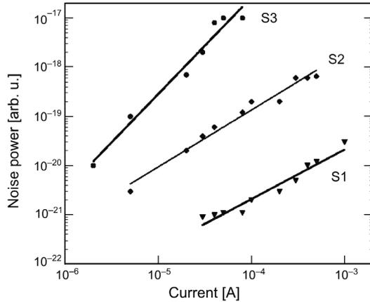
Fig. 7. Noise power density as a function of forward current at  $T = 77$  K and frequency  $f = 20$  Hz.
