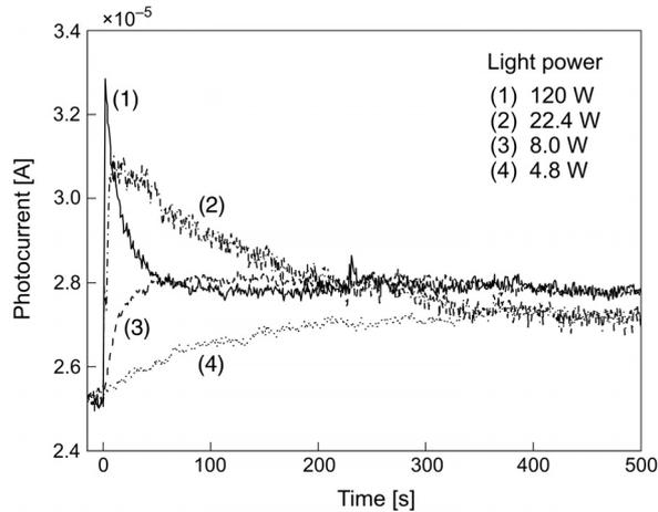
Fig. 5. Photocurrent versus time for various powers of the halogen lamp used to illuminate the sample.
