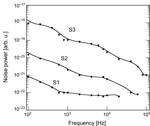
Fig. 6. Noise power density as a function of frequency at  $T = 77$  K and forward current  $I = 100 \mu\text{A}$ .
