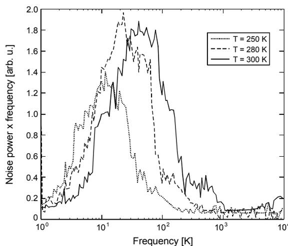
Fig. 8. Generation-recombination noise component obtained after multiplying the spectrum by the frequency  $f$  at various temperatures.
