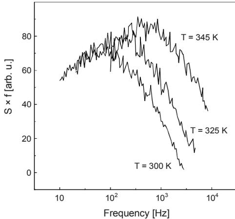
Fig. 1. Noise power density spectra at different temperatures.
