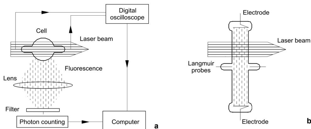
Fig. 2. Scheme of the experimental setup (a) and side view of the cell (b).
