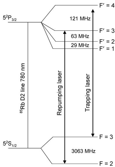
Fig. 1. Energy level diagram of the  $^{85}\text{Rb}$  atom. The hf structure of the  $D2$  line used in the cooling of  $^{85}\text{Rb}$  atoms is shown. Red detuned trapping laser and resonant repumping laser are marked by arrows.
