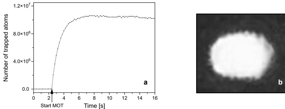
Fig. 6. Number of trapped atoms as a function of time elapsed from the switch on the trap – a. Image of the cloud of cold  $^{85}\text{Rb}$  atoms, as seen by CCD camera (its actual size is close to 1 mm, the picture was taken from the TV screen) – b.
