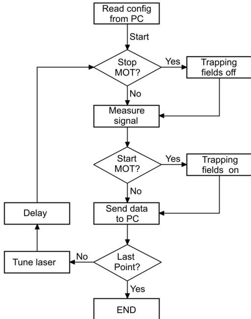
Fig. 5. The simplified flowchart of the main program of the microcontroller, steering the DMS200 system (a measurement on MOT with tuning laser wavelength).
