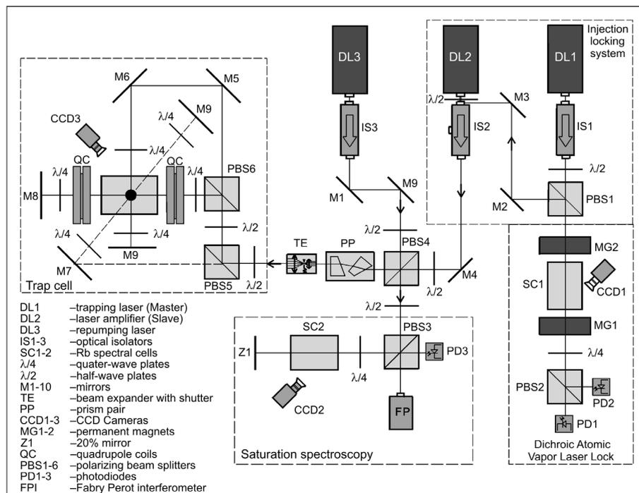
Fig. 2. General scheme of the magneto-optical trap. Essential blocks are marked with a dashed line.
