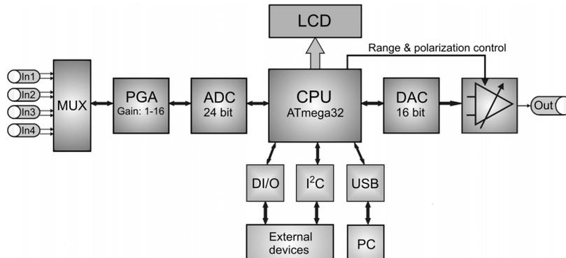
Fig. 4. Functional diagram of the DMS200 system for data acquisition, digital laser frequency tuning and control of the experiment: MUX – 4 channel analog multiplexer, PGA – programmable gain amplifier, ADC – 24 bit analog to digital converter, CPU – ATmega32 microcontroller, DAC – 16 bit digital to analog converter, DI/O – 4 digital output lines and 2 digital input lines,  $I^2C$  – two wire bus, USB – universal serial bus, LCD – 4 line LCD display.
