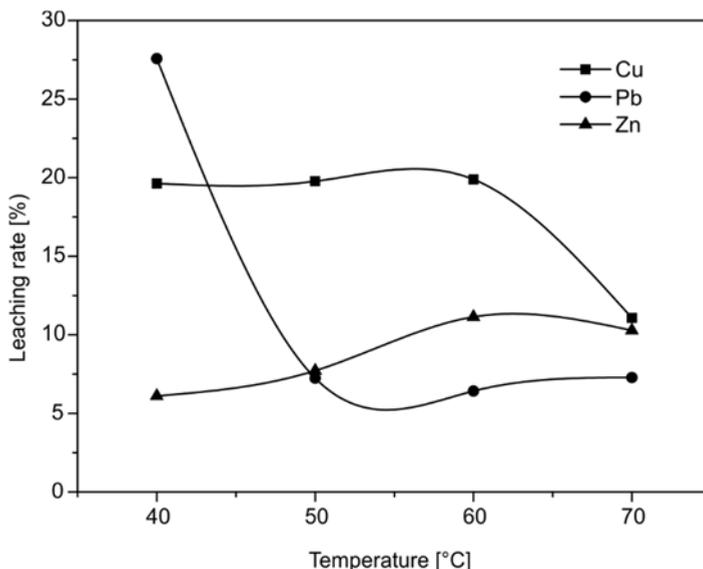
Fig. 5. Effect of temperature on the metal leaching rate (solid/IL ratio 1 g WPCBs/20 cm<sup>3</sup>, IL concentration 10 vol. %, H<sub>2</sub>O<sub>2</sub> dose 5 cm<sup>3</sup>/20 cm<sup>3</sup>, particle size 0.10–0.25 mm, leaching time 2 h)
