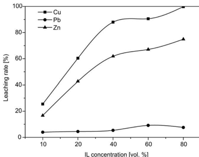
Fig. 2. Effect of IL concentration on the metal leaching rate (solid/IL ratio 1 g WPCBs/20 cm<sup>3</sup>, H<sub>2</sub>O<sub>2</sub> dose 5 cm<sup>3</sup>/20 cm<sup>3</sup>, particle size 0.1 to 0.25 mm, leaching temperature 50 °C, leaching time 2 h)
