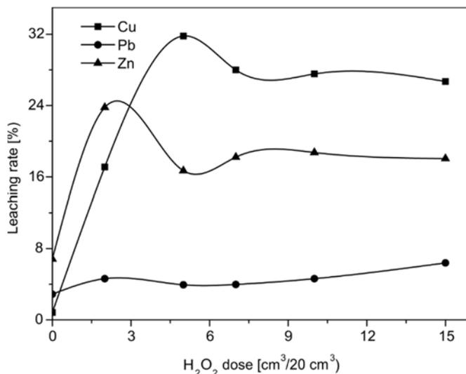
Fig. 3. Effect of H<sub>2</sub>O<sub>2</sub> dose on the metal leaching rate (solid/IL ratio 1 g WPCBs/20 cm<sup>3</sup>, IL concentration 10 vol. %, particle size 0.10 to 0.25 mm, leaching temperature 50 °C, leaching time 2 h)
