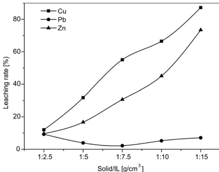
Fig. 4. Effect of solid/IL on metal leaching rate (IL concentration 10 vol. %, H<sub>2</sub>O<sub>2</sub> dose 5 cm<sup>3</sup>/20 cm<sup>3</sup>, particle size 0.10 to 0.25 mm, leaching temperature 50 °C, leaching time 2 h)
