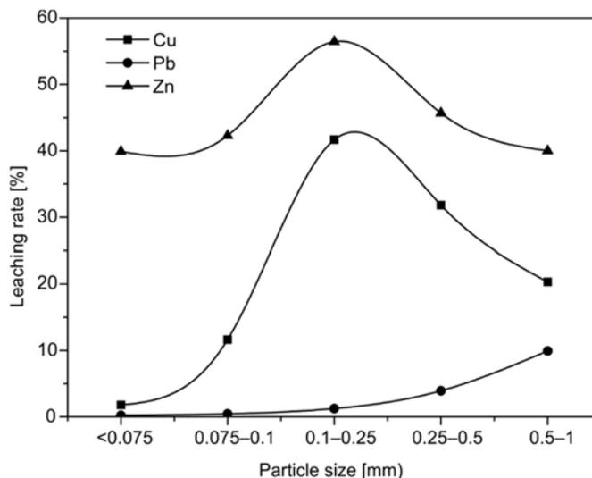
Fig. 1. Effect of particle size on the metal leaching rate (solid/IL ratio 1 g WPCBs/20cm<sup>3</sup>, IL concentration 10 vol. %, H<sub>2</sub>O<sub>2</sub> dose 5 cm<sup>3</sup>/20 cm<sup>3</sup>, leaching temperature 50 °C, leaching time 2 h)
