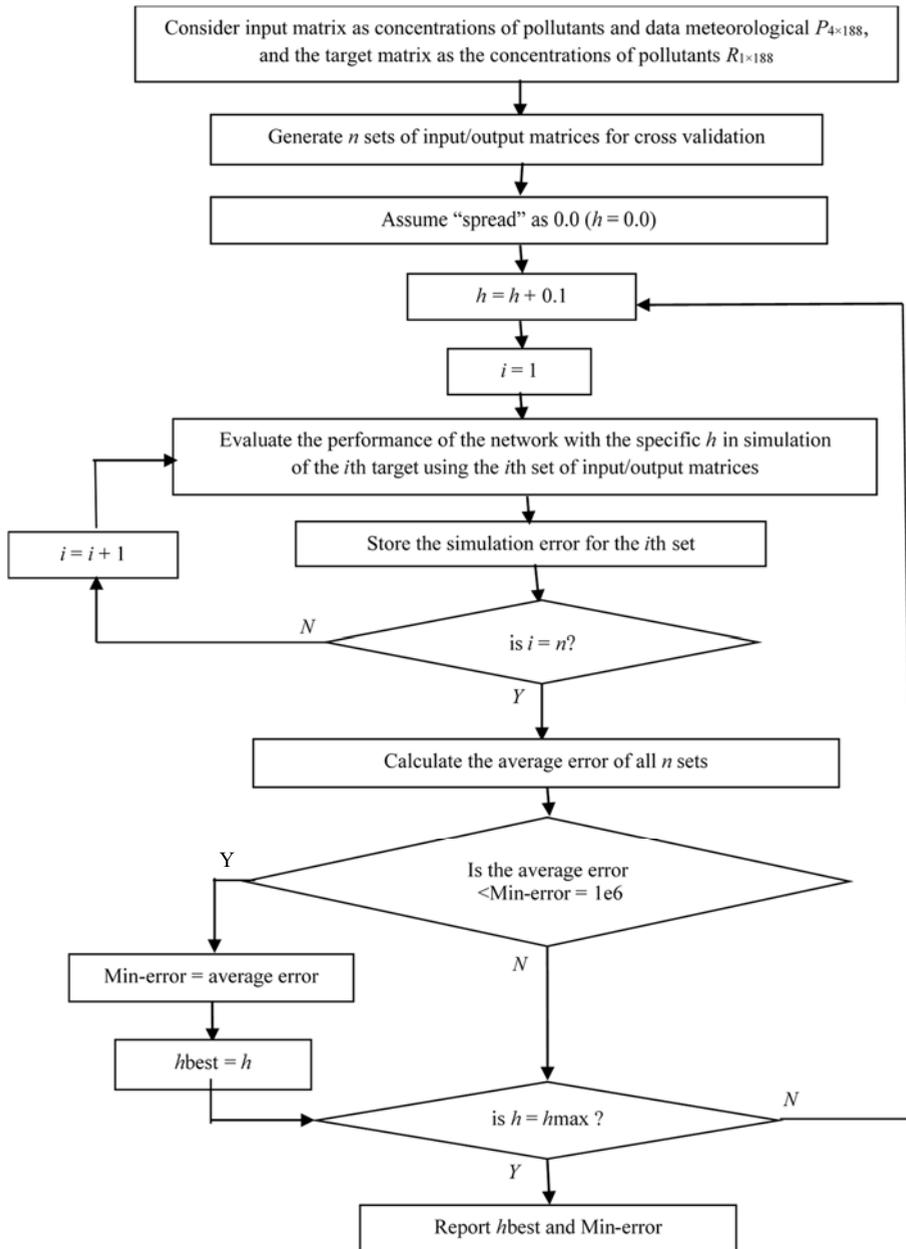
Fig. 3. Algorithm of the suitable spread ( $h$ )
