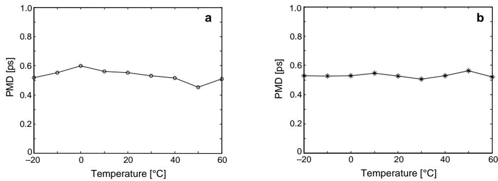
Fig. 4. Statistic PMD variance of FBG at varying temperature; temperature-compensated package (a) and unpackaged (b).
