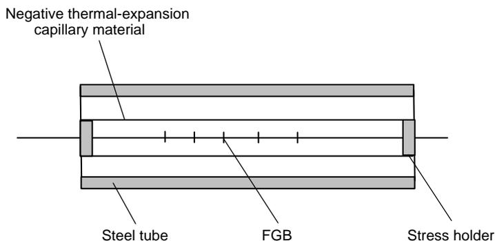
Fig. 1. Three-layer-structure package under tension for temperature-compensated FBG.
