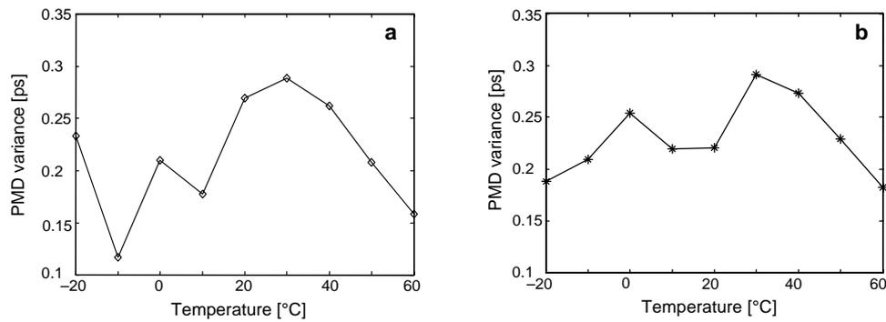
Fig. 5. Statistic PMD variance of FBG at varying temperature; temperature-compensated package (a) and unpackaged (b).
