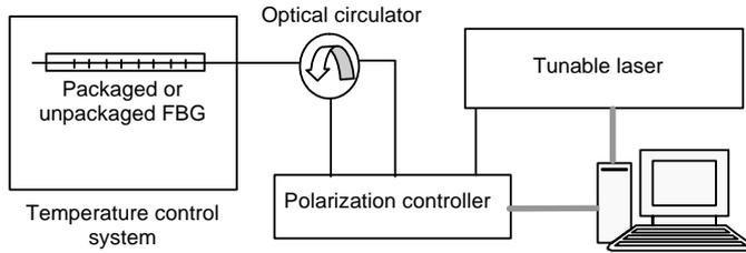
Fig. 3. Apparatus used for measurement of PMD of FBG with or without temperature-compensation using JME.
