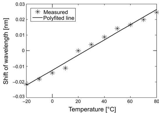
Fig. 2. Center wavelength shift of temperature-compensated FBG.
